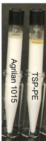
Figure 2. Stability comparison between Agrilan 1015 and TSP-PE after 2 weeks storage at 54 °C
