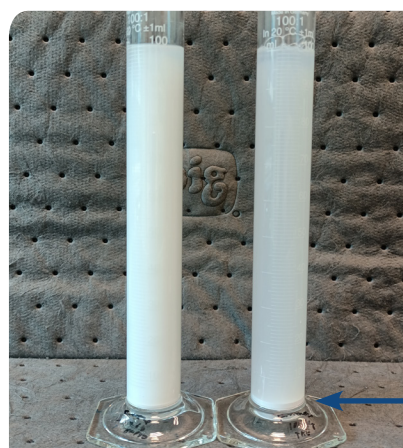
Left: Gly-IPA 480 SL 15% of Adsee AMP40 + Farnozine 900 WG Right: Gly-IPA 480 SL 15% of TAE + Farnozine 900 WG
