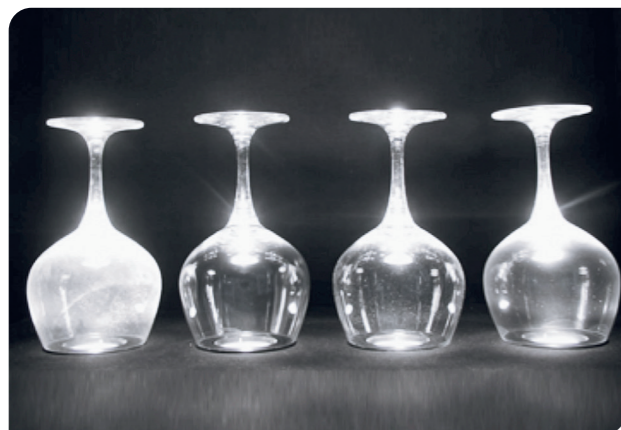
Figure 14: Anti-filming performance of a GLDA based ADW cleaner (2nd from left) containing Nouryon's Alcoguard® 4160-G polymeric co-builder after 30 washing cycles.
