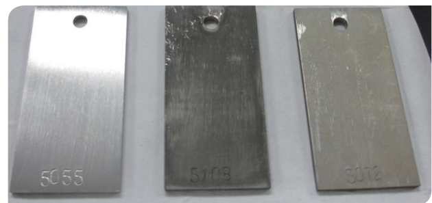
0.03% Armohib CI-28 0.03% JH-15 Blank 15% active hydrochloric acid, 6 hours soaking, RT 304 Stainless steel
