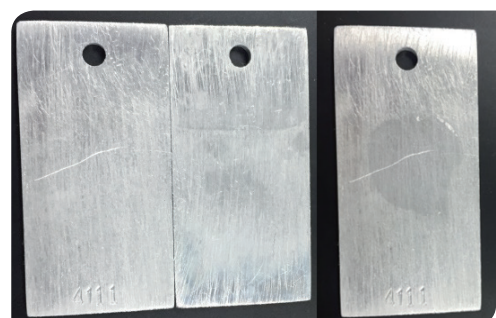
After washing: No corrosion is observed
