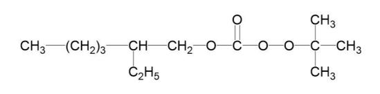
Trigonox® 117 can be used as initiator for the solution (co)polymerization of acrylates and methacrylates in the temperature range of 100-170°C, amongst others for the manufacture of coatings. Trigonox® 117 can also be applied as an initiator for the bulk and suspension (co)polymerization of acrylates and methacrylates.
