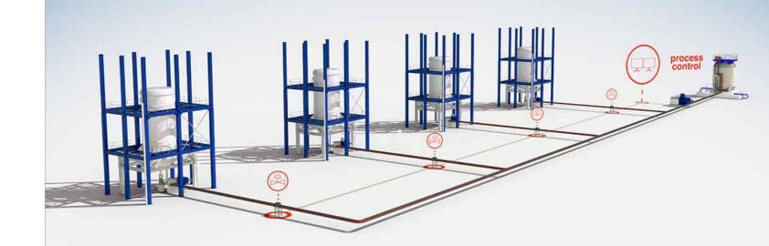
With CiD, the heat production in the reactor is controlled by the quantity of peroxide dosed throughout the polymerization process. To achieve this, fast peroxide, **Trigonox**<sup>®</sup> **187**, is used. As a result, the cooling capacity is optimized, and the batch time is reduced, increasing the overall capacity. The reaction can be stopped and restarted at any time by simply interrupting or restarting the peroxide
