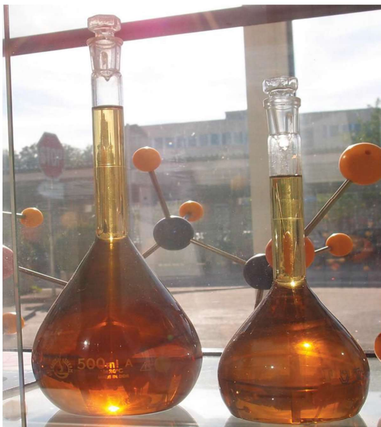
Liquid polysulfide polymers are light brown-colored polymers.
